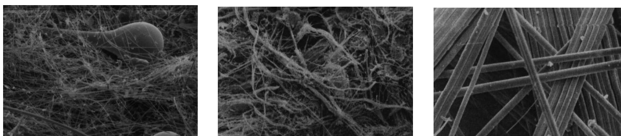
Figure 1 : microscopy of different fibres (mineral-250x, asbestos-500x, glass-250x)
