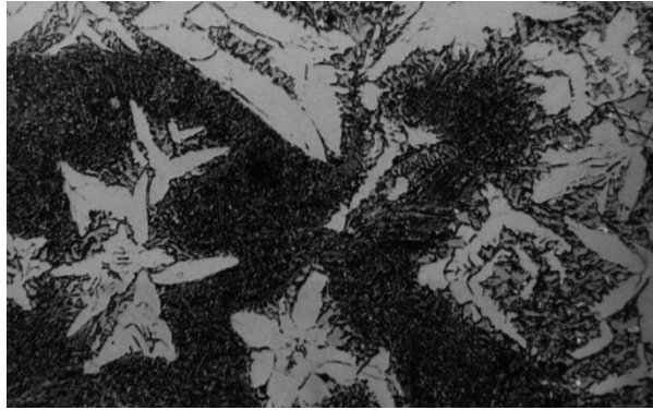
Figure 6 : microscopy of Melilite crystals in glassy matrix
